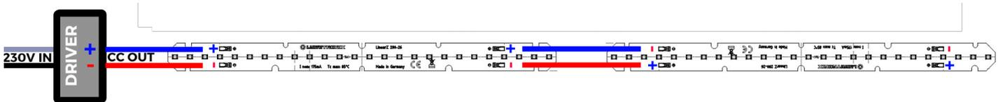
The series connection is applied by connecting the positive (+) terminal of the first LED strip to the negative (-) terminal of the second LED strip. This pattern is repeated for further LED strips, from the negative (-) of the second strip to the positive (+) of the third strip and so on. At the same time, the negative (-) of the first LED strip is wired to the (+) of the second, then the (-) of the second to the (+) of the third and so on.
