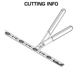
The LED strip can be separated or shortened every 45.45 mm. The connectors work on the separated parts also.
