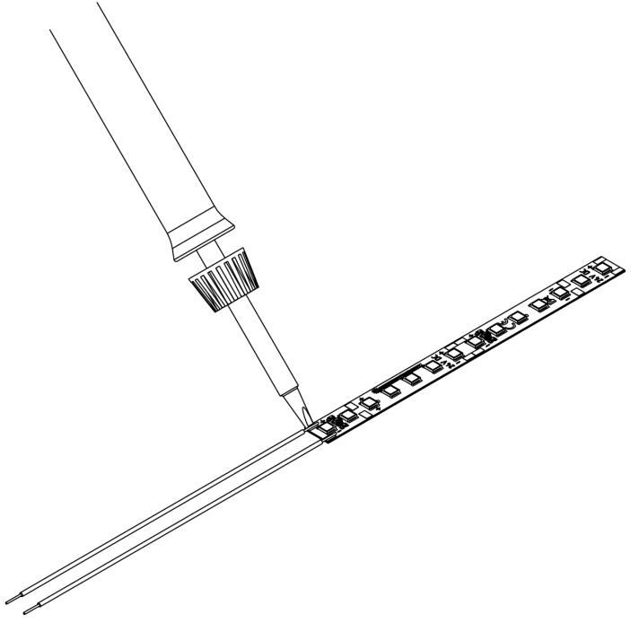
The Professional LED Strips are connected via a lead connection to the connection pads provided for this purpose.
