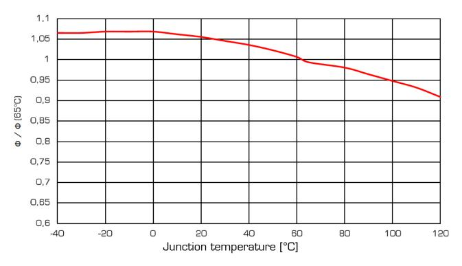
LUMINOUS FLUX vs. TEMPERATURE
