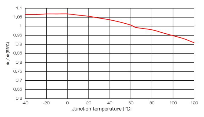
LUMINOUS FLUX vs. TEMPERATURE
