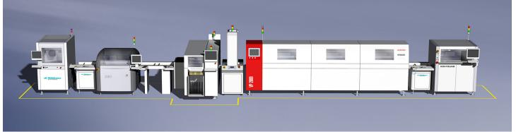
This LED module is made on a ISO-certified production line that has been tailored specifically to the requirements of assemblies with LED technology. Nearly one million components can be processed per day in the production line.
