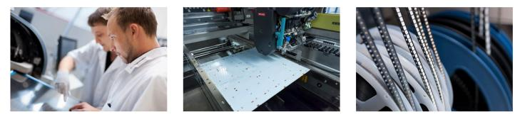
The MatrixMini is **made in Germany**, at a production line that uses the innovative manufacturing technology of plasma direct metallization, to turn substrates into electrical conductive and solderable circuit boards, even those that before have not been suitable for an assembly with electronic components.
