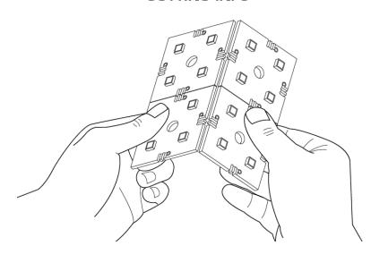
The LED module can be separated into smaller units up to 1 single module of 30x30mm. The connectors work on the separated parts also.
