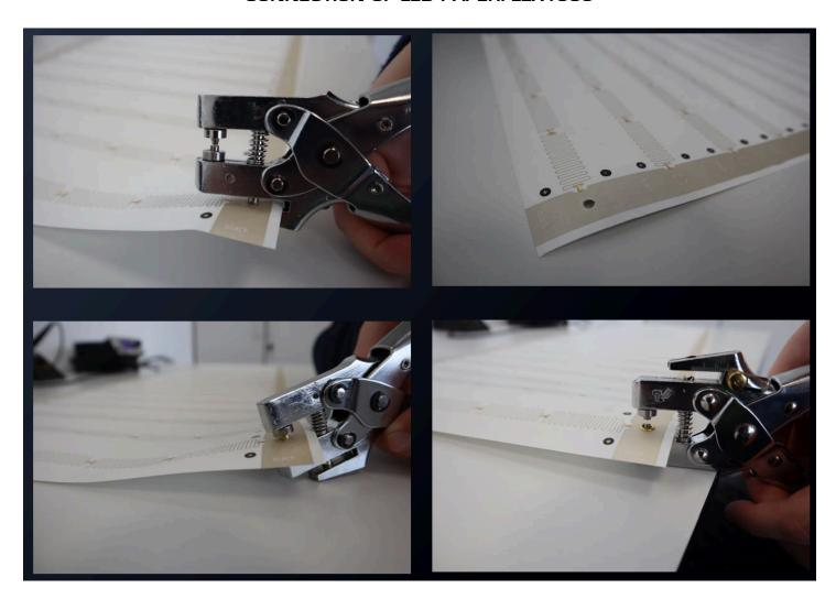
The PaperFlex1080 can be connected to wires via a Eyelet Pliers tool, such as found here: <a href="https://www.conrad.de/de/search.html?search=BGS%20technic%20%C3%96senzange">https://www.conrad.de/de/search.html?search=BGS%20technic%20%C3%96senzange</a>
