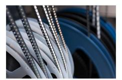
This LED strip is **made in Germany**, at a flex production line that uses the innovative manufacturing technology of plasma direct metallization, to turn flexible substrates into electrical conductive and solderable circuit boards, even those that before have not been suitable for an assembly with electronic components.
