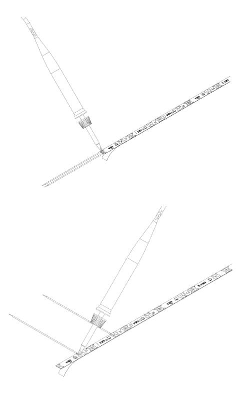
The Professional LED Strips are connected via a lead connection to the connection pads provided for this purpose.
