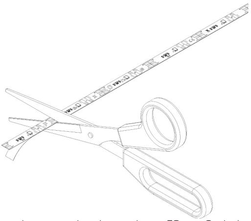
The LED strip can be separated or shortened every 50 mm. On the back of the LED strip is a double-sided heat-conducting adhesive tape, which allows installation of the LED strip. Professional LED strips can be cut with scissors.
