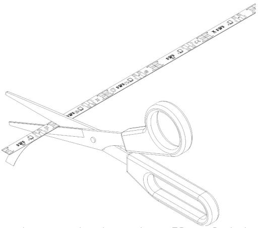
The LED strip can be separated or shortened every 50 mm. On the back of the LED strip is a double-sided heat-conducting adhesive tape, which allows installation of the LED strip. Professional LED strips can be cut with scissors.
