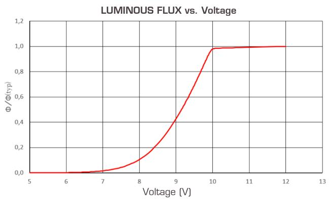
Due to the special conditions in the production process of LEDs, the specified values are statistical averages. The individual LED may deviate from them.
